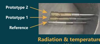
**Radiation & temperature** resistant HN connector up to 600 °C
