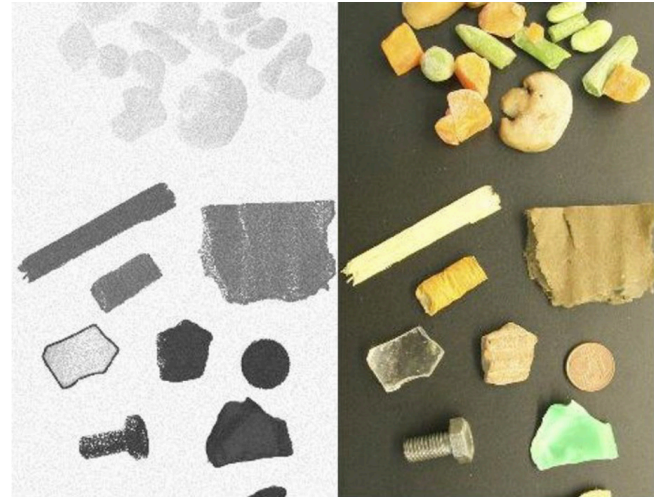
Fig. 2. In the visible light image (right) an assortment of frozen vegetables (top) has similar shapes and colors to various types of packaging and other debris. In the SWIR image (left) the foodstuffs absorb the IR wavelengths while the debris reflects it, leading to a strong contrast between the two. (Image courtesy of Tomra.)
