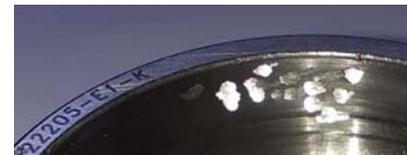
**Figure 3. Intentionally pre-damaged outer raceway**
