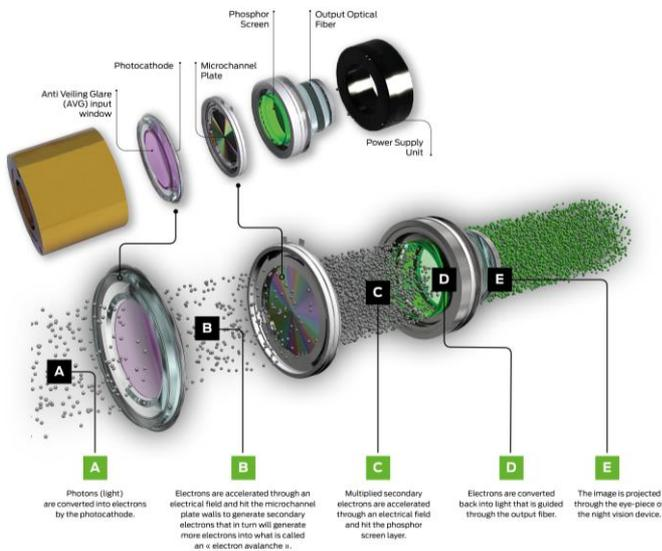
This is the key (engine) component of any night vision device.
