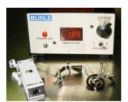
Model PF1053 is a solid-state, bench-top High Voltage Power Supply that can provide an output of up to +/- 3 kV dc and 1 mA. The output polarity can b e set to negative or positive via the front pa nel switch. This model offers high precision and stability in a compact, economical package which makes it ideal for many laboratory applications.
