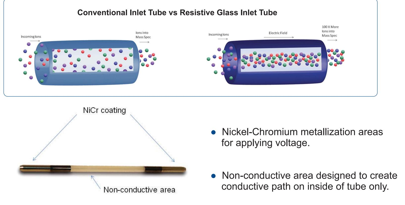
Typical Single Capillary Tube shown with an OD of 6.5 mm and an ID of 0.6 mm
