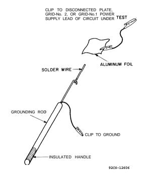
Figure 3 - Suggested Arrangement for Effectiveness Test of Protective Devices During Steady-State Operating Conditions
