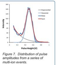
Figure 7. Distribution of pulse amplitudes from a series of multi-ion events.
