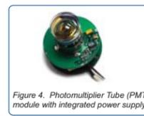
Figure 4. Photomultiplier Tube (PMT) module with integrated power supply.
