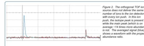
Figure 2. The orthogonal TOF ion source does not deliver the same number of ions to the ion detector with every ion push. In this ion push, the isotope peak is present while the main peak (which is on average ~14 times more abundant) is not. The averaged signal (blue) shows a waveform with the proper abundance ratio.
