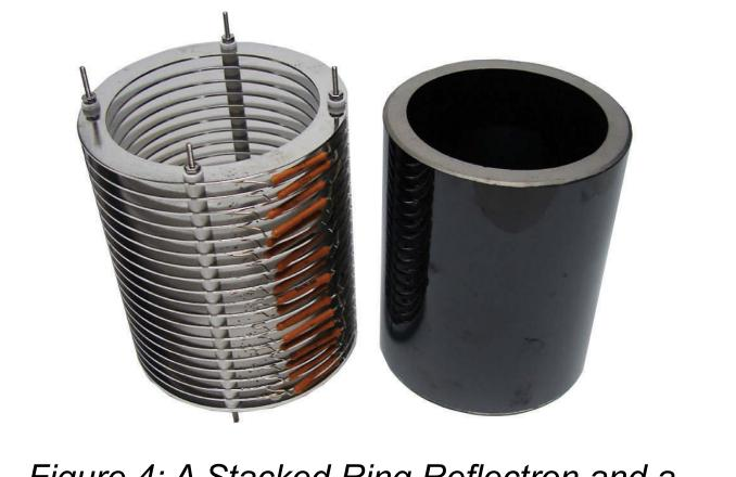
Figure 4: A Stacked Ring Reflectron and a Resistive Glass Reflectron side-by-side.
