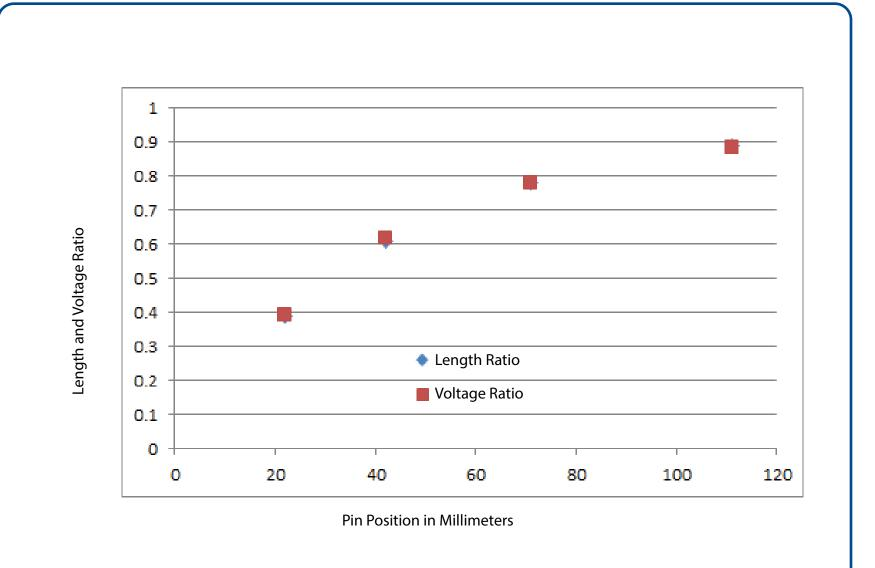
Figure 9: The graph indicates pin position in millimeters, and shows a good correlation between the position of the pins and the measured voltage.
