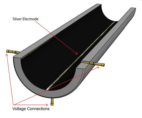
Figure 10: Cross section of a Resistive Glass Tube configured as a collision cell or ion guide.
