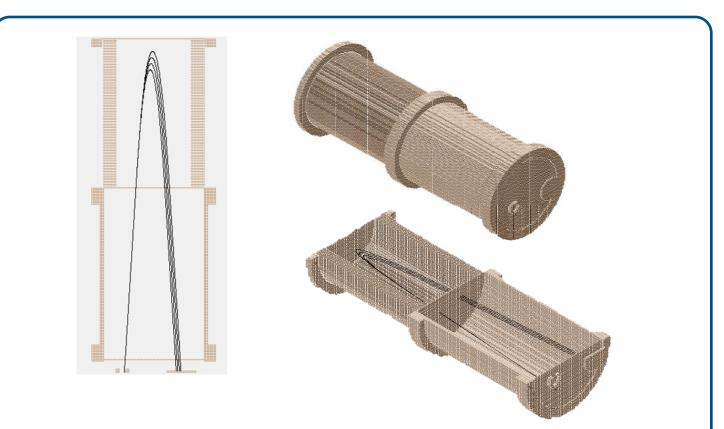
Figure 3: A Diagram of a Reflectron Lens.
