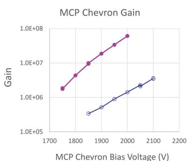
Figure 2: Increase in Chevron-MCP detector gain due to MCP coating
