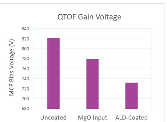
Figure 5: Effect on QTOF tune voltage
