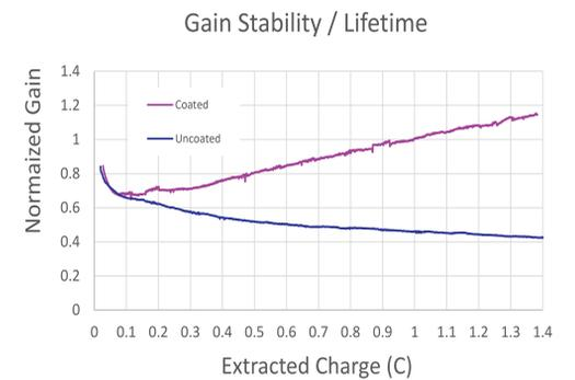
Figure 3: Relative gain as a function of extracted charge for coated and uncoated Chevron-MCP detectors
