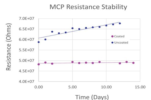
Figure 4: Resistance stability of coated and uncoated MCPs exposed to atmosphere
