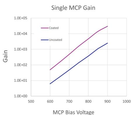
Figure 1: Single MCP Gain before and after coating
