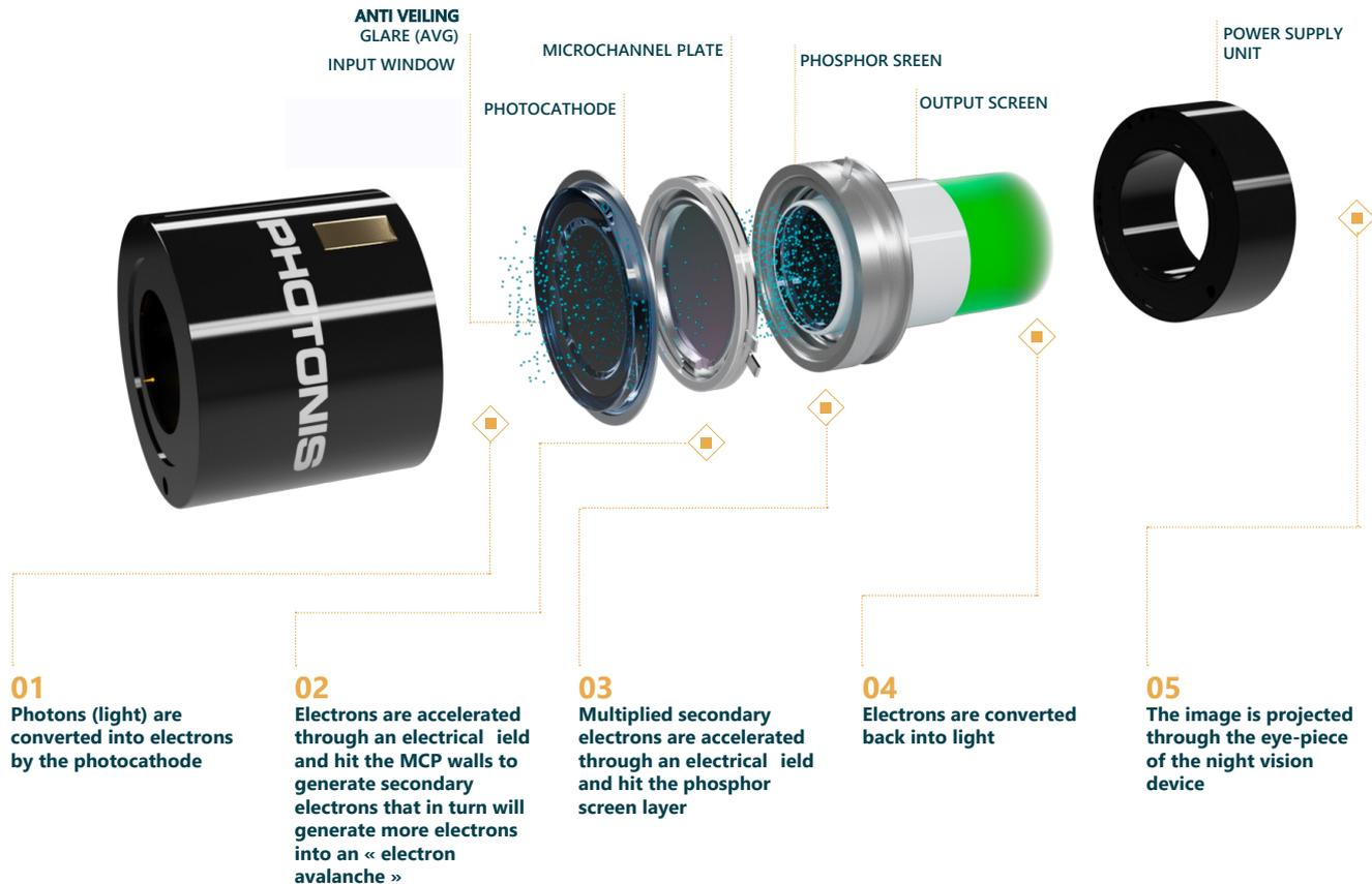
The MCP is a thin glass disc, less than a half a millimeter thick, which contains millions of small channels. When an electron coming from the photocathode strikes the inner wall of one channel, several secondary electrons are generated by the impact. Each of these secondary electrons will be accelerated
