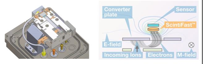
Fig 2. (Left) “Agate” detector prototype (photo). (Right) Principle of operation
