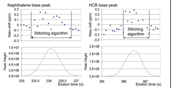
Fig 10. GC MS, Megamix 1ng load, 1000 shots per spectrum (800 high gain, 200 low gain). Elution on Naphthalene (left) and HCB (right). Mass shift due to the algorithm is below 0.5ppm. Internal calibration by PFTBA leak signal is applied after stitching algorithm.
