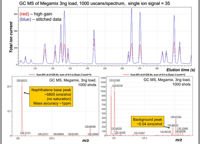
Fig 7. GC MS, Megamix 3ng load, 1000 shots per spectrum (800 at high gain, and 200 at low gain). (Top) Comparison between stitched ion signal and raw ion signal (high gain). (Bottom) Intense peak (left) and minor peak (right) in the same spectrum of naphthalene at maximum of eluted GC peak.
