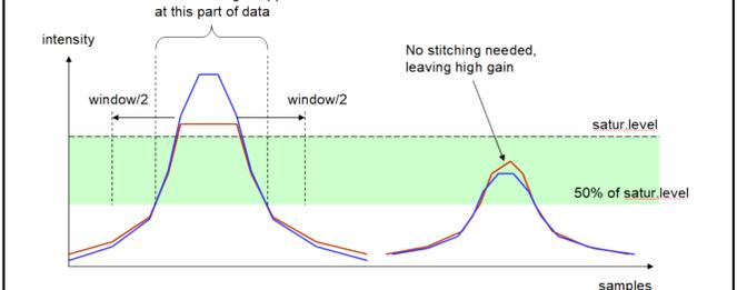
Fig 6. Stitching explanation. (Left) Peak height above saturation level – recording a weighted sum of high and low gain signals. (Right) Peak height is below saturation level – high gain signal is recorded.
