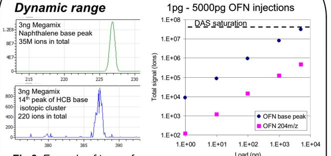
Fig 8. Example of traces for intense (left) and minor (right) ion peaks. Fig 9. Test of DR by OFN injections.
