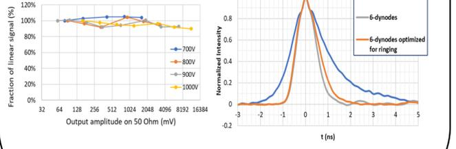
Fig 3. (Left). Linear detector (6-dynodes) respond up to 10V (Right) Detector time respond is below 1ns.
